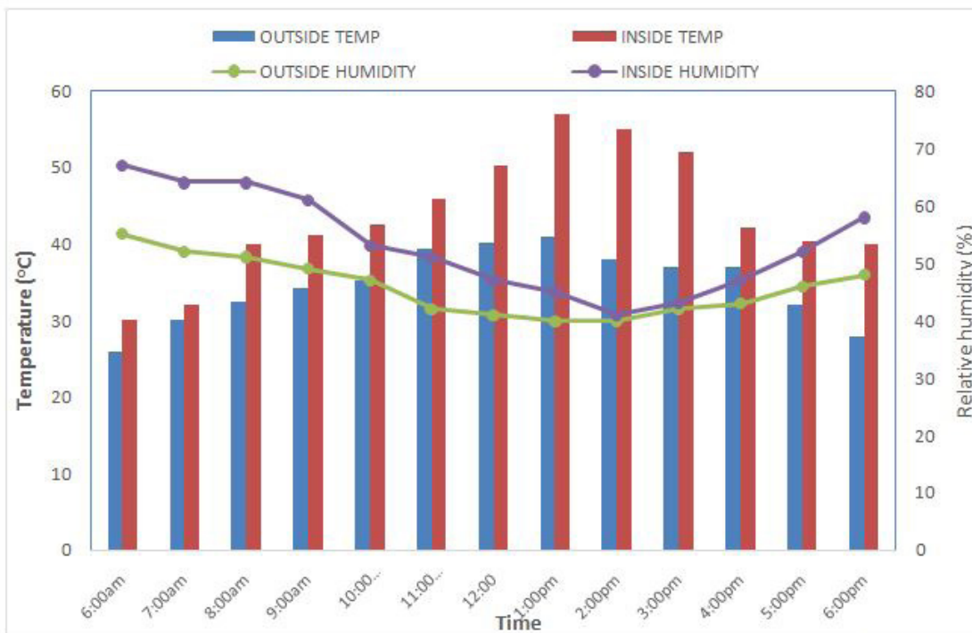
Fig. 2 Average temperature and relative humidity inside greenhouse during 14 th week
