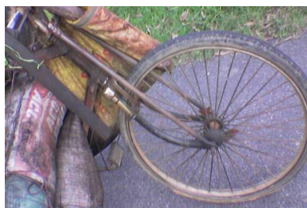
Figure-2. The wheel is replaced with cycle rickshaws' stouter wheel & spokes
