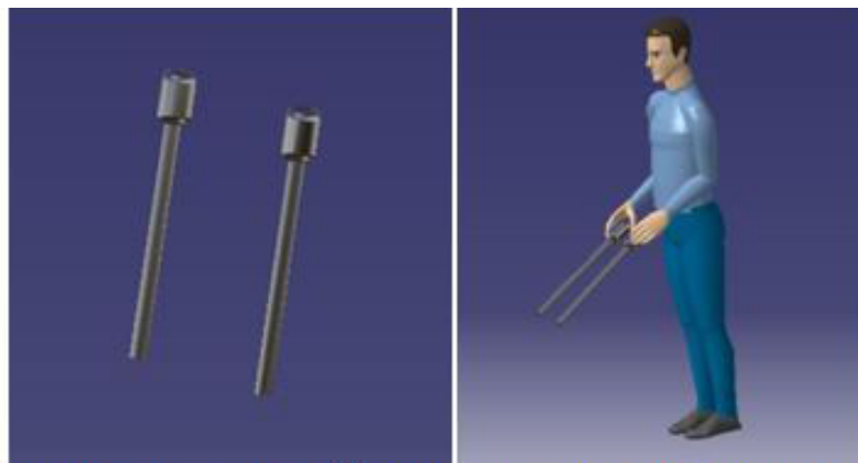
HANDLES WITH A 50 th Percentile MALE MANICKIN SHOWING THE HAND GRASP STRUCTURE OF A COOLIE IN THE HOWRAH STATION
