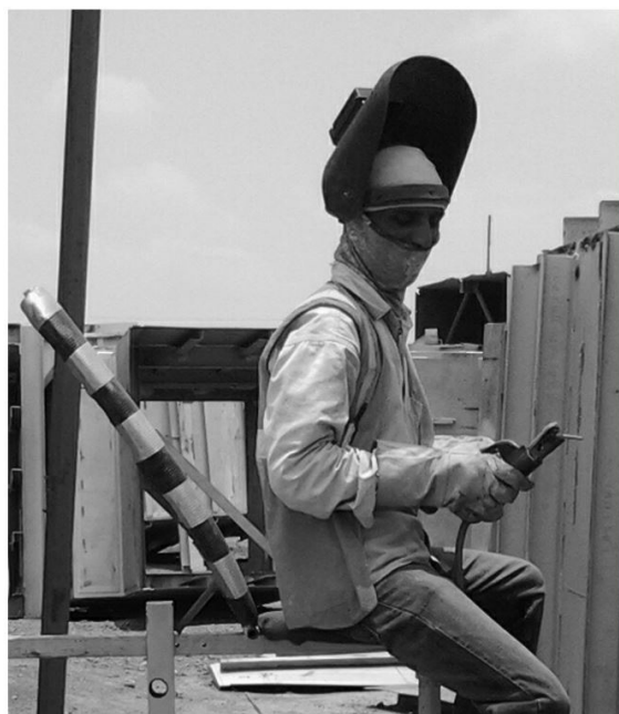
Fig. 1 This is the complete view of the welders chair. The sitting part, the central iron beam, the circular base, the foot rest are clearly visible.
