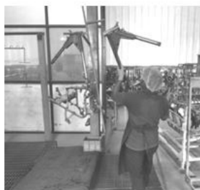
Figure.4 Shot blasting stage of vehicle frame
